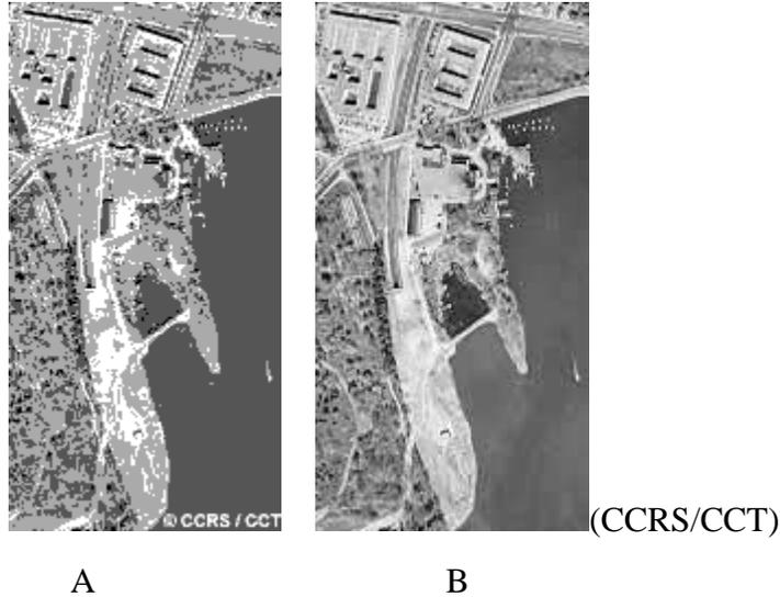
Image B has a higher radiometric resolution, or a higher bit rate than image A. This is apparent by the increased number of shades of grey reducing the 'blocky-ness' found in image A with its inability to distinguish different intensities as well as the higher resolution system that produced image B.
